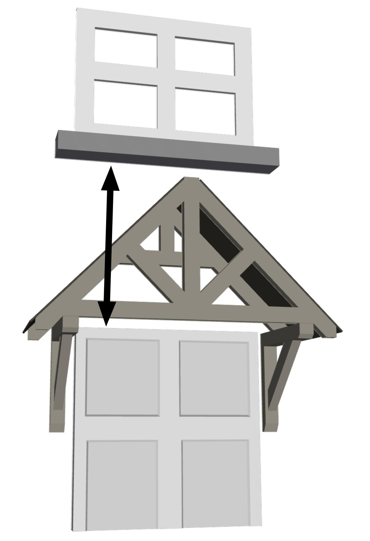
Measure the height between your door and any restrictions above (e.g. windows, guttering)
